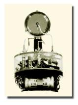
come variable between omni through cardioid to figure-8 maintaining a practically constant sensitivity. The power supplies for the model M 49 microphones included a potentiometer with a pointer knob and a corresponding scale.
